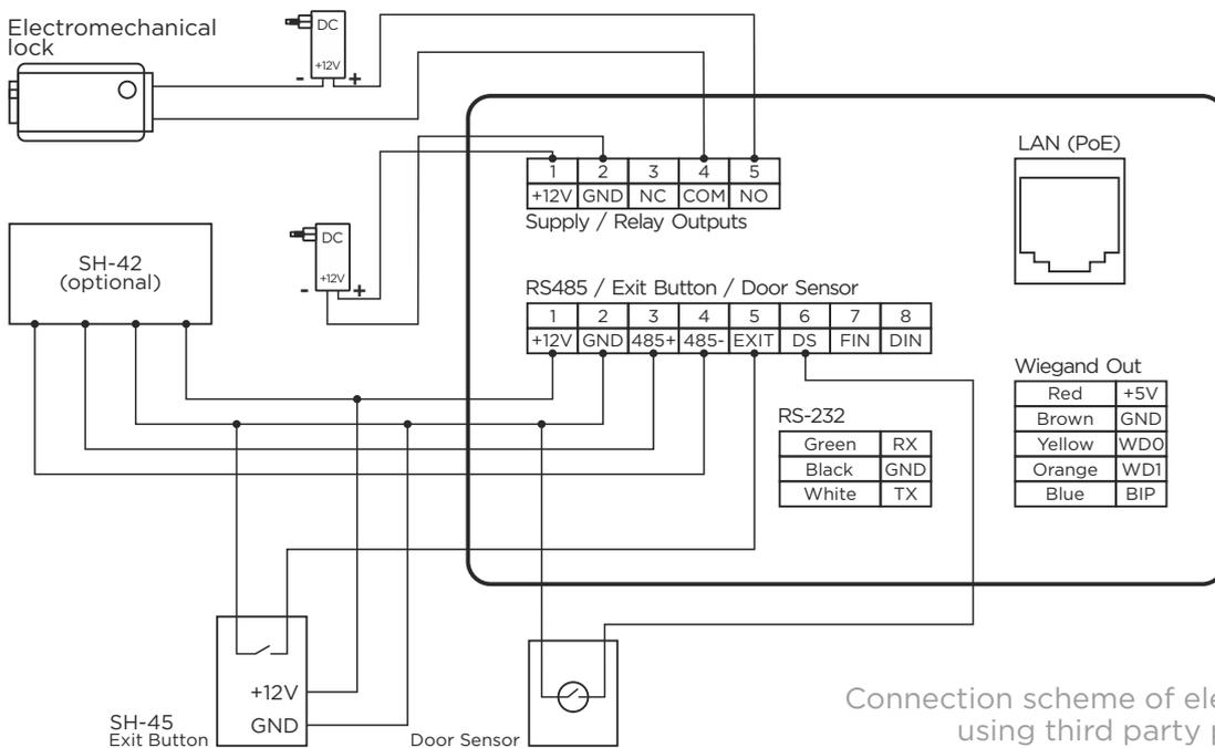
Connection scheme of electromechanical lock using third party power supply
