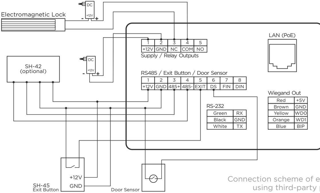
Connection scheme of electromagnetic lock using third-party power supply
