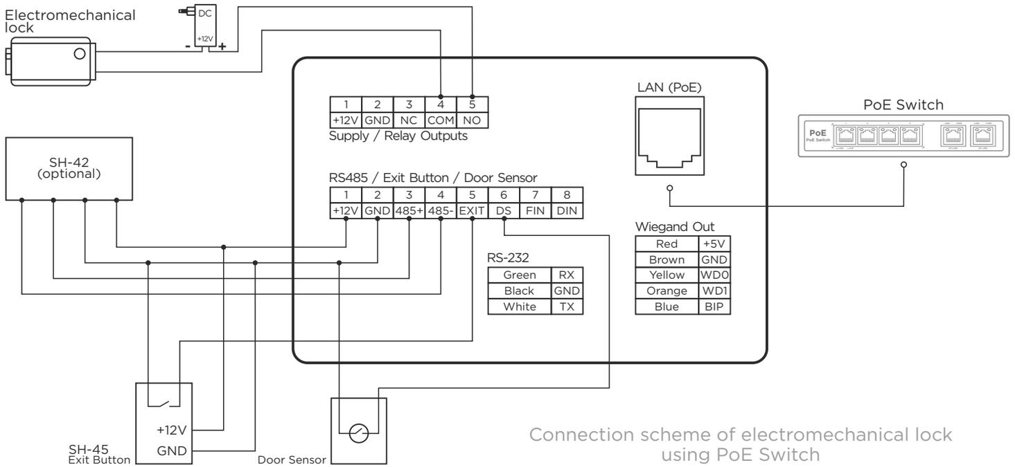
Connection scheme of electromechanical lock using PoE Switch
