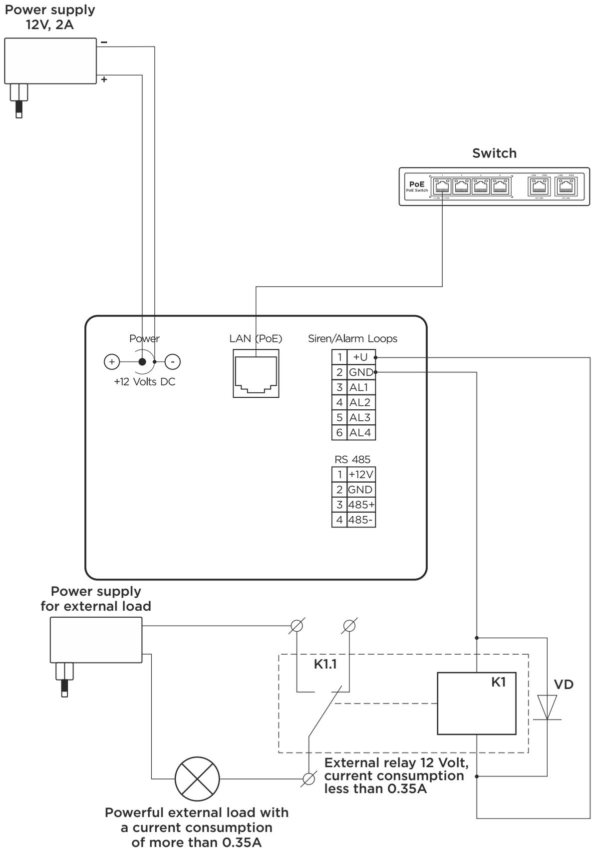
Scheme for connecting external controlled devices or connecting a powerful external load to the siren output using an external additional relay
